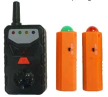
Receiver has 4 different corresponding LED light indicators that correspond to the same LED light / transmitter when a fish strikes
